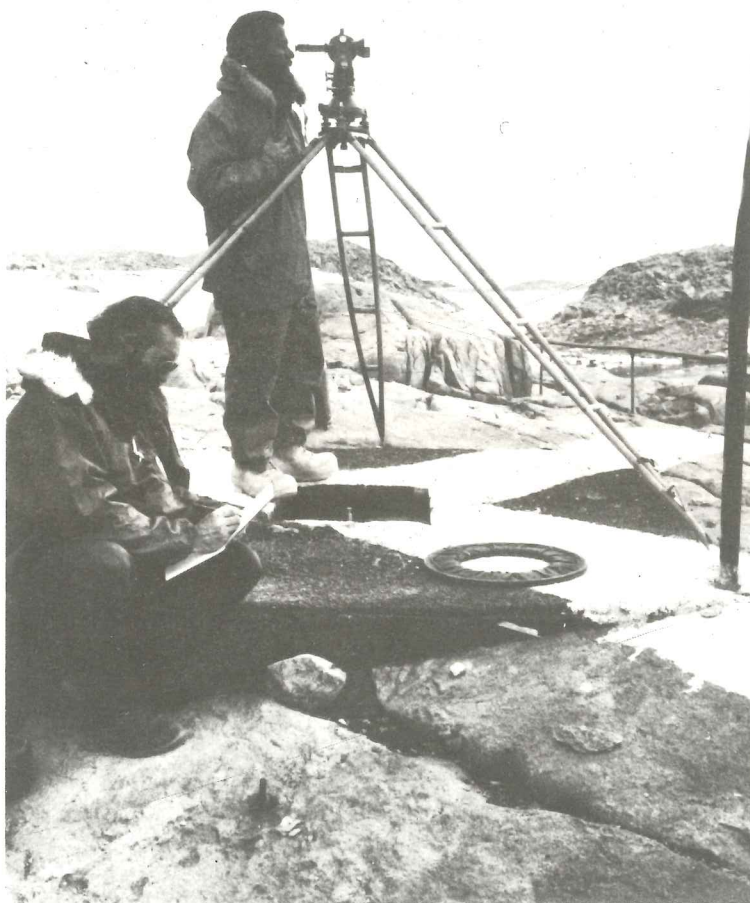
Plate 5 Triangulation work on the Pageos site using a Wild T3 theodolite.
